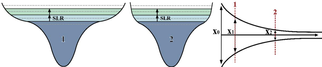
**Figure 1: Schematic display of SLR in estuary cross-sections (left) and schematic plan view of an estuary (right). For two cross-sections with large (1) and small (2)  $S_{INT}$ . The cross-sections show the MW as black lines for a reference scenario (dark blue), and two SLR scenarios (light blue and light green).**
