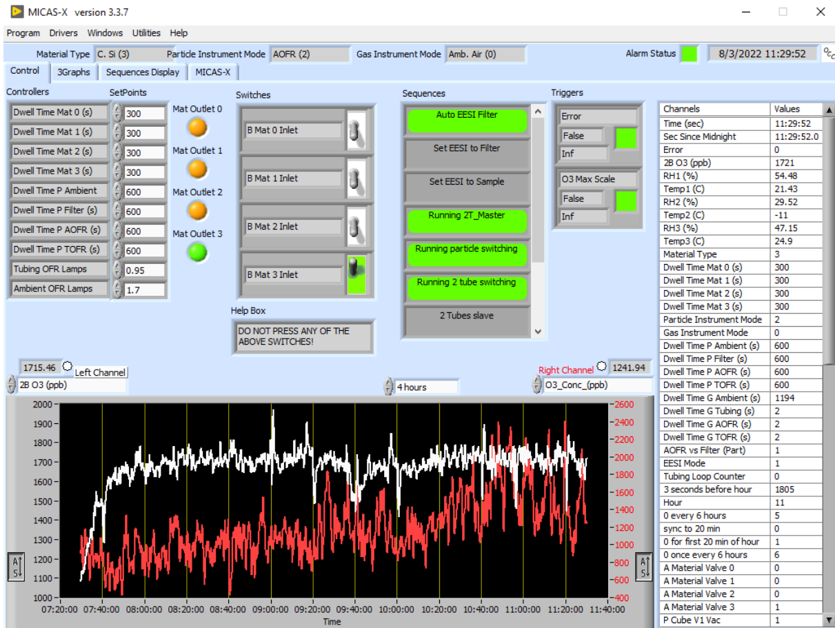
Figure S1. Screenshot of the custom user interface for the GVS acquisition software (MICAS, Original Code, Boulder, CO) within Labview. The user can control the GVS valves manually, set a dwell time for each polymer inlet, or code a more complex valve switching sequence.
