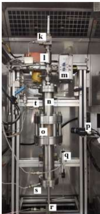
90 Figure 4 The inside-view of the air bath:(k)Hopper valve; (l) Proppant warehouse; (m) Electric valve of proppant warehouse; (n) Up chamber of the sapphire reactor; (o) Sapphire window of the sapphire reactor; (p) Camera; (q) Strain sensor; (r) Pore pressure valve and safety valve; (s) Stress valve; (t) Temperature sensor.
