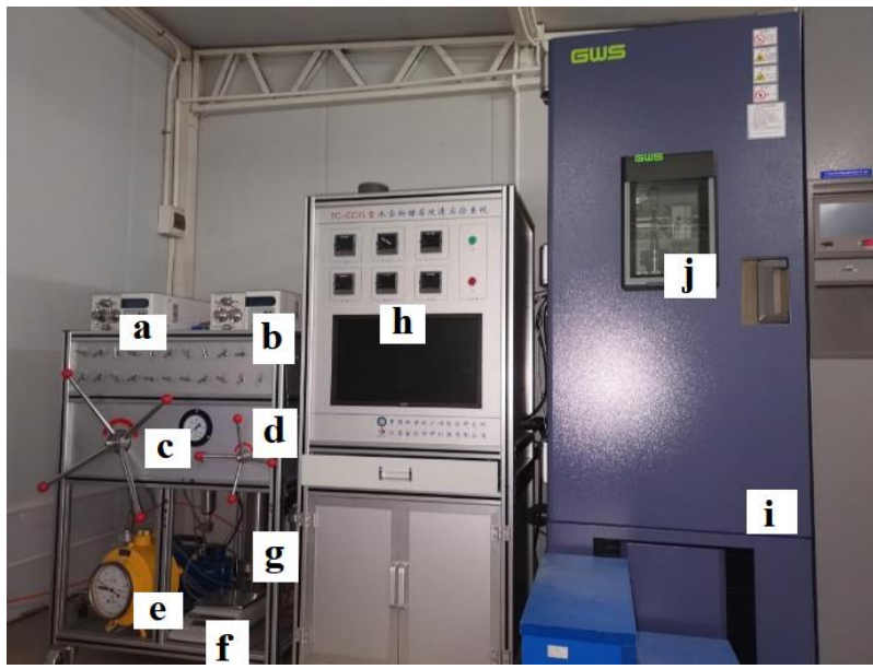
85 Figure 3 The front view of the apparatus: (a) Fracturing pump (b) Pore pressure pump (c) Overlying stress (d) Back pressure pump (e) Wet type gas flowmeter (f) Electronic balance (g) Separator (h) Control cabinet and computer (i) Air bath (j) Visual window of air bath and sapphire reactor
