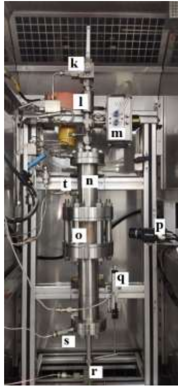
90 Figure 4 The inside-view of the air bath:(k)Hopper valve; (l) Proppant warehouse; (m) Electric valve of proppant warehouse; (n) 95 Up chamber of the sapphire reactor; (o) Sapphire window of the sapphire reactor; (p) Camera; (q) Strain sensor; (r) Pore pressure valve and safety valve; (s) Stress valve; (t) Temperature sensor.
