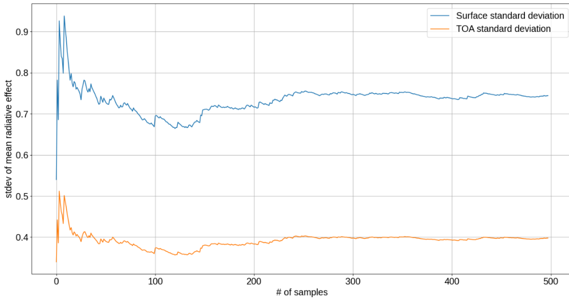
Figure 6: Standard deviation of the histogram shown in Figure 5 as a function of the number of samples that make up the perturbed parameter ensemble for a given set of optical property uncertainties.
