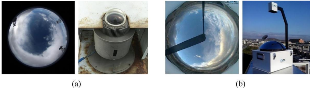
42 Figure 1: Two kinds of ground-based cloud images and their observation equipment: (a) ASI ground-based cloud image 43 and its observation equipment (Cazorla et al., 2008; Shi et al., 2019); (b) TSI ground-based cloud image and its observation 44 equipment (Long et al., 2006).
