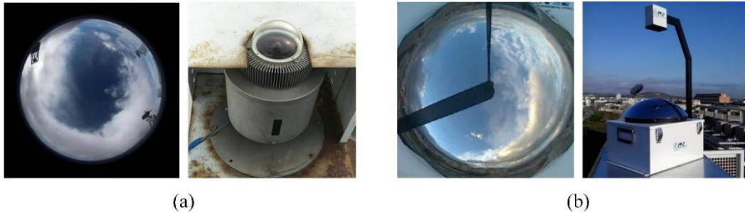
41 42 Figure 1: Two kinds of ground-based cloud images and their observation equipment: (a) ASI ground-based cloud image 43 and its observation equipment (Cazorla et al., 2008; Shi et al., 2019); (b) TSI ground-based cloud image and its observation 44 equipment (Long et al., 2006).
