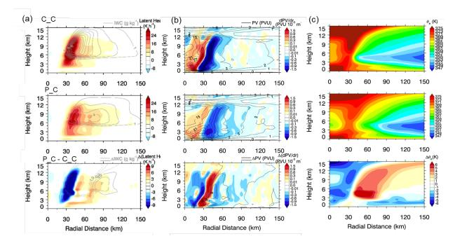
Figure 10. Vertical-radial cross-sections of 20-hr (32–52 hour) azimuthal means of (a) latent heat overlaid with ice water content (IWC), (b) equivalent potential temperature ( $\theta_e$ ), and (c) potential vorticity (PV) and its gradient for C\_C, P\_C case, and their difference (P\_C - C\_C) from top to bottom.
