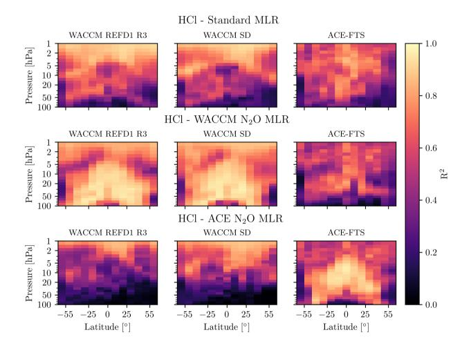
Figure A4. Goodness of fit for ACE-FTS and WACCM HCl. Top row:  $R^2$  for standard MLR. Centre row:  $R^2$  for WACCM N<sub>2</sub>O MLR. Bottom row:  $R^2$  for ACE-FTS N<sub>2</sub>O MLR.
