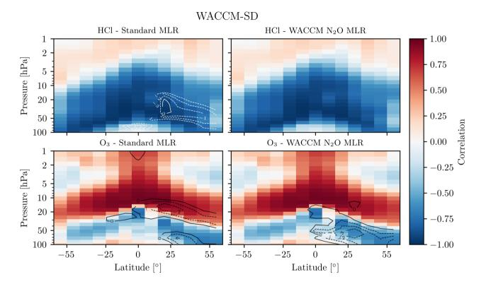
Figure 5. Top row: correlation coefficient for WACCM-SD HCl and  $N_2O$ . White contours show where the HCl trend is greater than -3%/decade. Bottom row: correlation coefficient for WACCM-SD  $O_3$  and  $N_2O$ . Black contours show where the  $O_3$  trend is less than 0%/decade. The trend contours in the left row were calculated with the standard MLR, and the trend contours in the right row were calculated with the N<sub>2</sub>O MLR.
