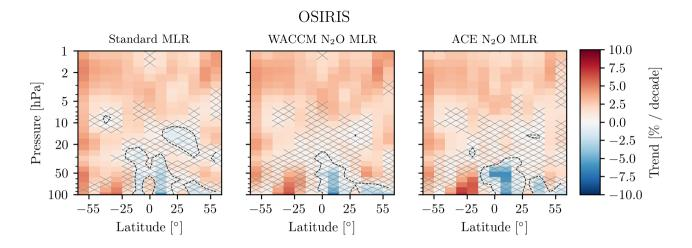
**Figure 6.** OSIRIS  $O_3$  trends for 2004/02 – 2018/12. Hatched regions are insignificant at the  $2\sigma$  level. Dashed contours mark the transitions from positive to negative trends.
