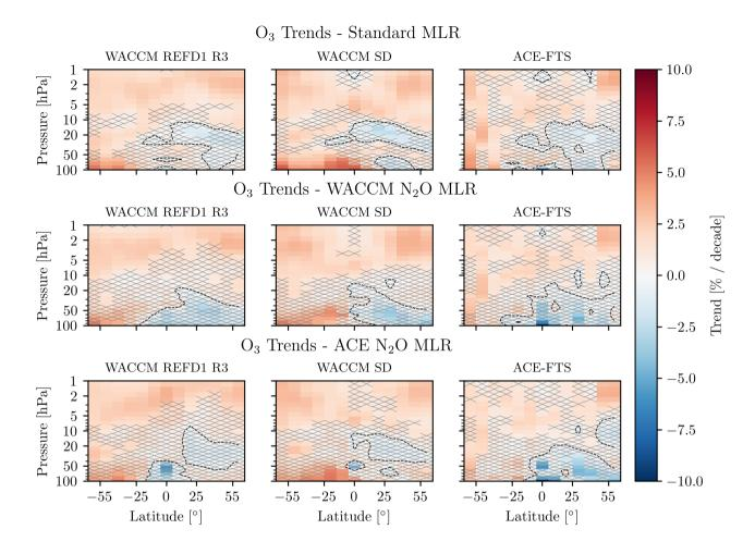
Figure 4.  $O_3$  trends for 2004/02 – 2018/12. Top row: trend calculated with standard MLR. Centre row: trends calculated with WACCM  $N_2O$  MLR. Bottom row: trends calculated with ACE-FTS  $N_2O$  MLR. Hatched regions are insignificant at the  $2\sigma$  level. Dashed contours mark the transitions from positive to negative trends.
