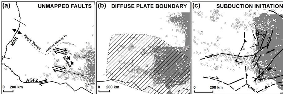
**Figure 5.** Schematic cartoons to illustrate the different hypothesis on the origin of seismicity of the WIM. a) shear corridors, inverse transform faults b) diffuse plate boundary c) initiation of subduction.
