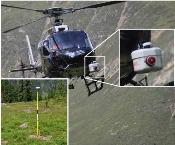
191 Figure 3: ALS data collection on 08.08.2019 in Horlachtal. Helicopter with nose-mounted VP1 laser scanner as well as the ground 192 station which recorded the dGNSS raw data during the flight time (Stonex S9III).
