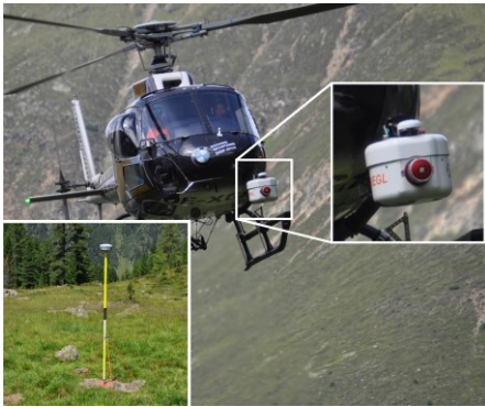
Figure 3: ALS data collection on 08.08.2019 in Horlachtal. Helicopter with nose-mounted VPI laser scanner as well as the ground station which recorded the dGNSS raw data during the flight time (Stonex S9III).
