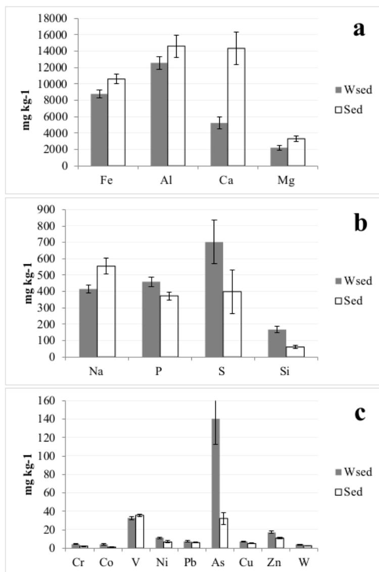
245 **Figure 6 – Concentration of elements and heavy metals in the sediments of Bolsena lake. (a) Elements originated from the lithological substrate; (b) elements of mixed origin; (c) Heavy metals (natural and/or anthropogenic sources).**
