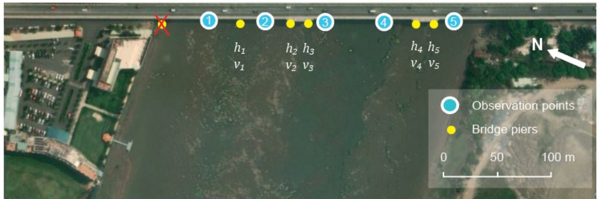
Figure R1. Bridge piers considered, and representation of flow velocity ( v ) and water depths ( h ) upstream of each pier i . The bridge pier marked with a red cross was not considered as likely to have scour holes. Copyright: Bing Maps.
