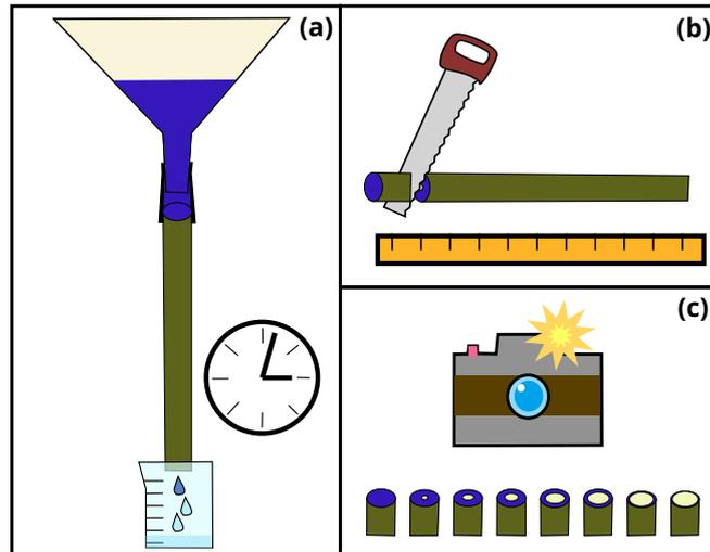
**Figure 1.** Sketch to illustrate the steps of the dye tracer experiment: (a) Application of dye tracer to stem segment; (b) Cutting the stem into smaller sub-segments; (c) Capturing images of cut surfaces for each sub-segment
