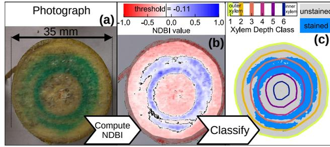
**Figure 2.** Exemplary images for the processing of cut surface #15. (a) shows the original photograph, (b) shows the computed NDBI values overlain by a mask that excludes everything but the xylem and (c) shows the detected blue stained area (light blue pixels) within six xylem depth classes.
