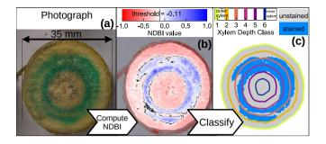
Figure 2. Exemplary images for the image-processing of cut surface #15. (a) shows the original photograph, (b) is shows the respective xylem-computed NDBI values overlain by a mask that excludes everything but the xylem and (c) shows the detected blue stained area (light blue pixels) within six xylem depth classes (outer borders depicted by dark blue to yellow circles).
