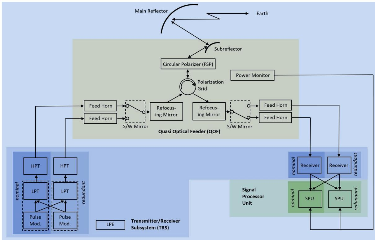
**Figure 11.** Simplified block diagram of CPR.
