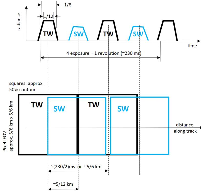
**Figure 21.** BBR: Schematic of the SW and TW acquisition sequence. This is for the nominal Chopper Drum speed. However, in order to maximise the life time of the Chopper Drum, it is considered to operate the Chopper Drum at 75% of the nominal speed, which leads to a respective stretch of the sequences. The resulting performance of in integrated 10 km × 10 km pixel will remain within required specification. (Courtesy of Thales Alenia Space, UK.)
