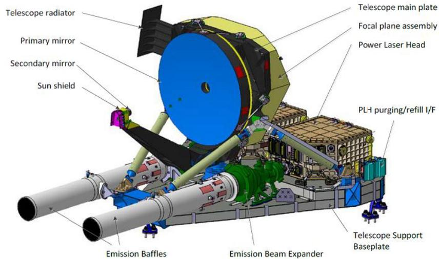
**Figure 3.** Illustration of ATLID bistatic architecture. This graphic representation shows the two fully redundant transmitting chains including their emission telescopes. The long emission baffles at the exit of the two laser heads minimise risk of LIC for the exit windows. (Courtesy of Airbus DS, France.).
