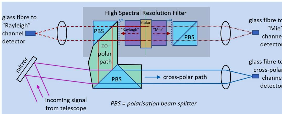
**Figure 5.** ATLLID receiver optical path schematic. Returned signal collected from the telescope is passing through a Polarisation Beam Splitter and the total cross polar signal is separated to the cross polar path (via fiber, to end up in the cross polar channel detector). The remaining co-polar signal enters the HSR filter, that separates the Mie from the Rayleigh in individual polar channels.
