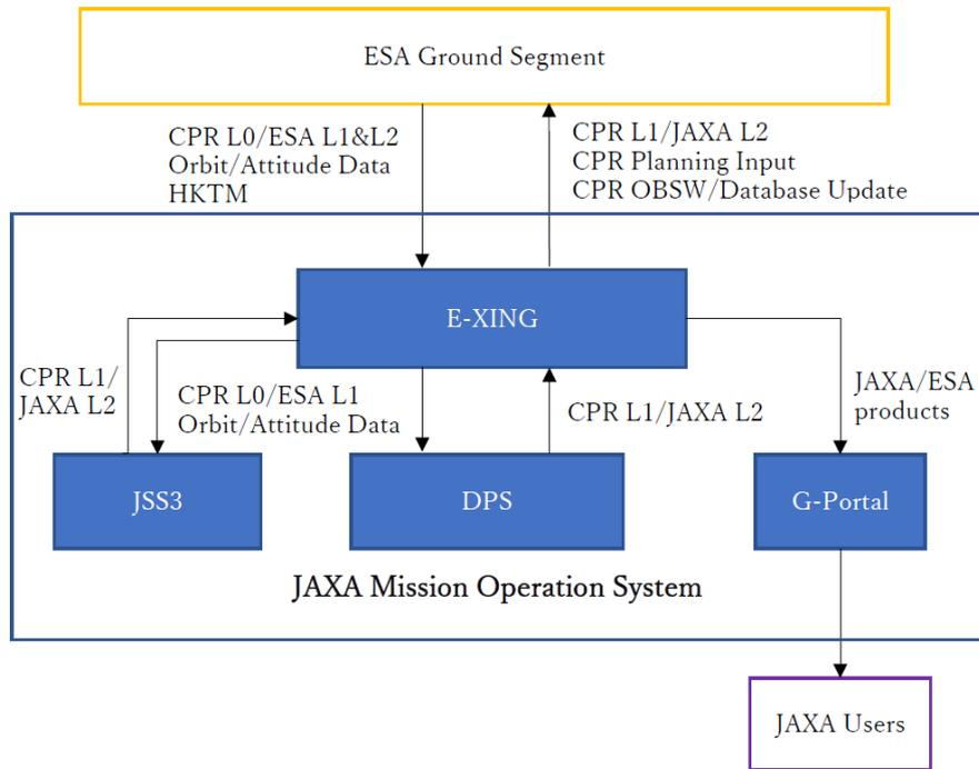
**Figure 24.** Components of JAXA mission operation system.
