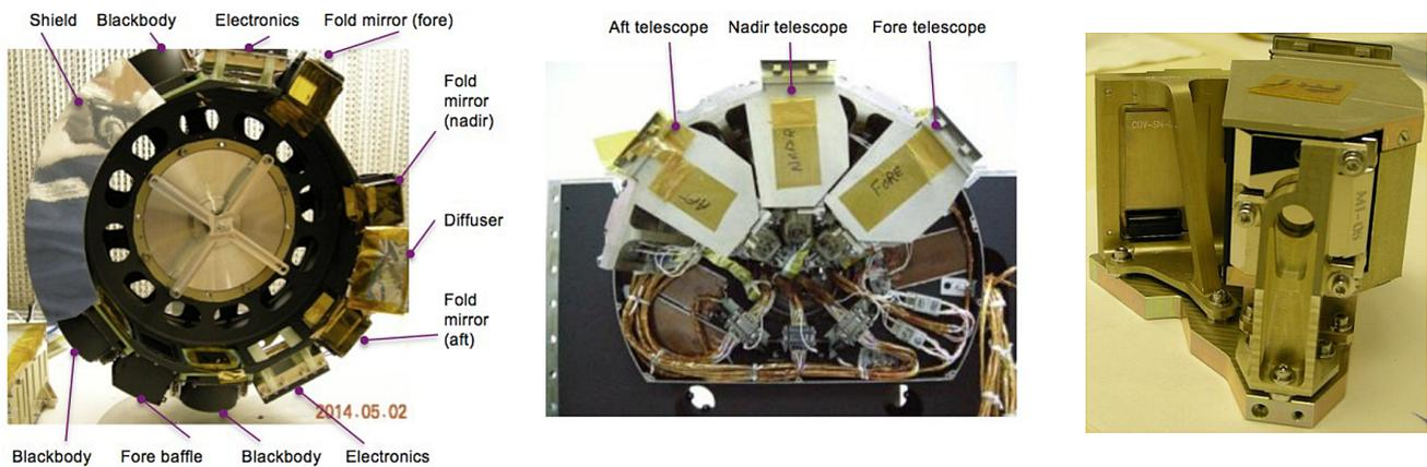
**Figure 19.** BBR Calibration Drum (left), Telescope Baseplate Assembly (centre) and photograph of one individual telescope (right). The nadir and aft baffles and one blackbody are hidden behind the shield of the Calibration Drum. (Courtesy of STFC RAL Space, UK.)
