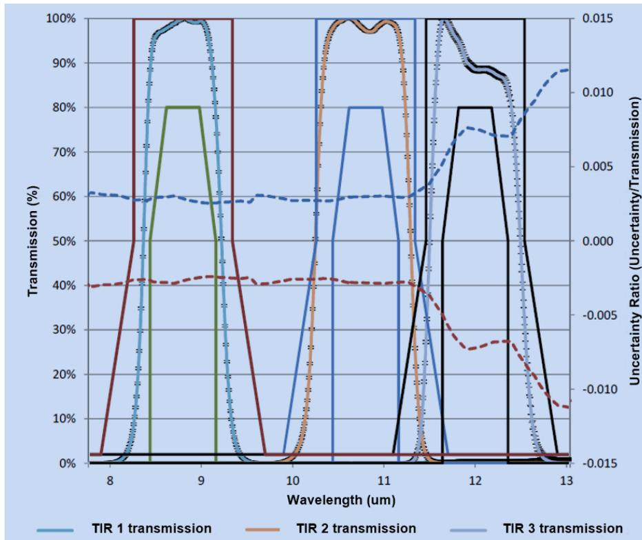
**Figure 17.** MSI TIR filter functions. The filter function requirements are indicated by the solid lines (TIR 1: red and green, TIR 2: blue, TIR 3: black). The dashed lines indicate the  $3\sigma$  uncertainties on the transmission values (red: low reference signal, blue: high reference signal, according to Table 4). (Courtesy of SSTL, UK.)
