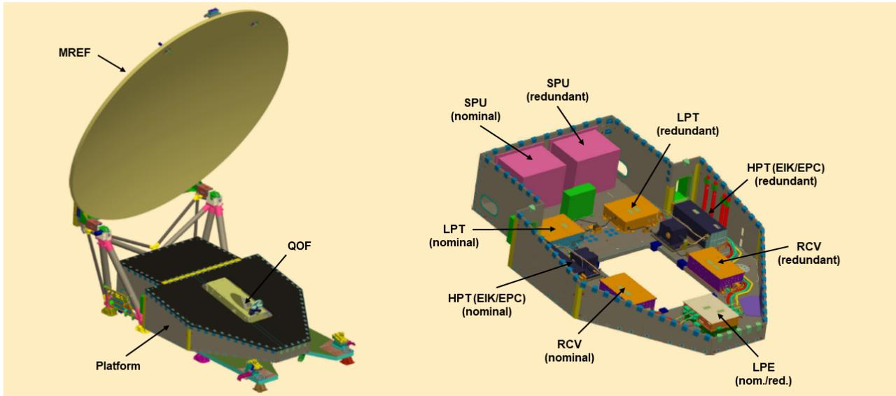
**Figure 10.** CPR external view with MREF deployed (left) and major components layout inside Platform with upper panel opened (right). (Courtesy of NEC)
