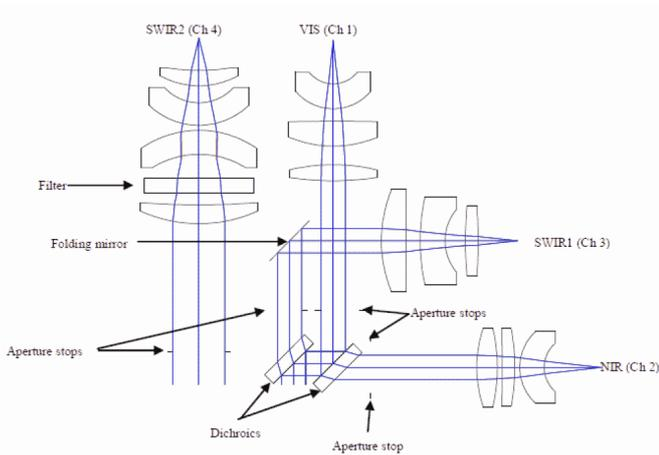
**Figure 13.** MSI VNS optical layout. (Courtesy of SSTL, UK.)
