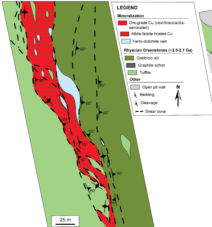
855 Figure 6: A) A mine level map at 300 m of the Southern Pahtohavare deposit showing albite felsite hosted Cu in a structurally-controlled position. The construction of the mine level map was done for resource estimates during the 1990s by utilizing vertical cross sections from profiles every ten meters along the strike of the ore body with 3 to 5 inclined drillholes in each profile intersecting the ore body at various depths. Geological contacts and structures have been interpolated from the vertical cross sections. Dipping of contacts and structures are estimated from the cross sections and are not based on actual structural measurements. B) The Southeastern Pahtohavare open pit showing both the stratabound and discordant ore zones. Structural measurements were acquired during mapping in the 1990s. 860
