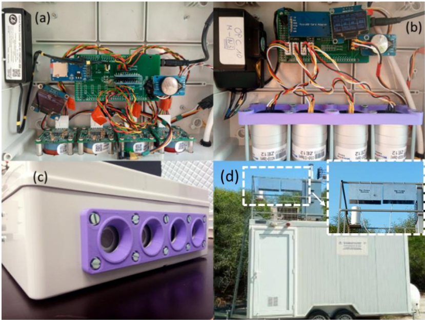
Figure 1: Images showing the layout of the AQ monitors housing the Alphasense (a) and the Winsen (b) LCSs, the side of the AQ monitors at which the sensing elements of the LCSs were exposed to the ambient air (c), and the place that the AQ monitors were installed at the top of the reference station (d).
