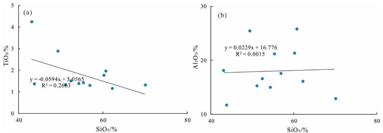
Figure.9 Intersection diagram of TiO<sub>2</sub> and SiO<sub>2</sub> (a) and intersection diagram of Al<sub>2</sub>O<sub>3</sub> and SiO<sub>2</sub> (b)
