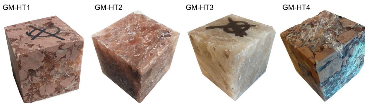
Figure 2: The four cubes of rock salt (60x60x60 mm) before experimental deformation.
