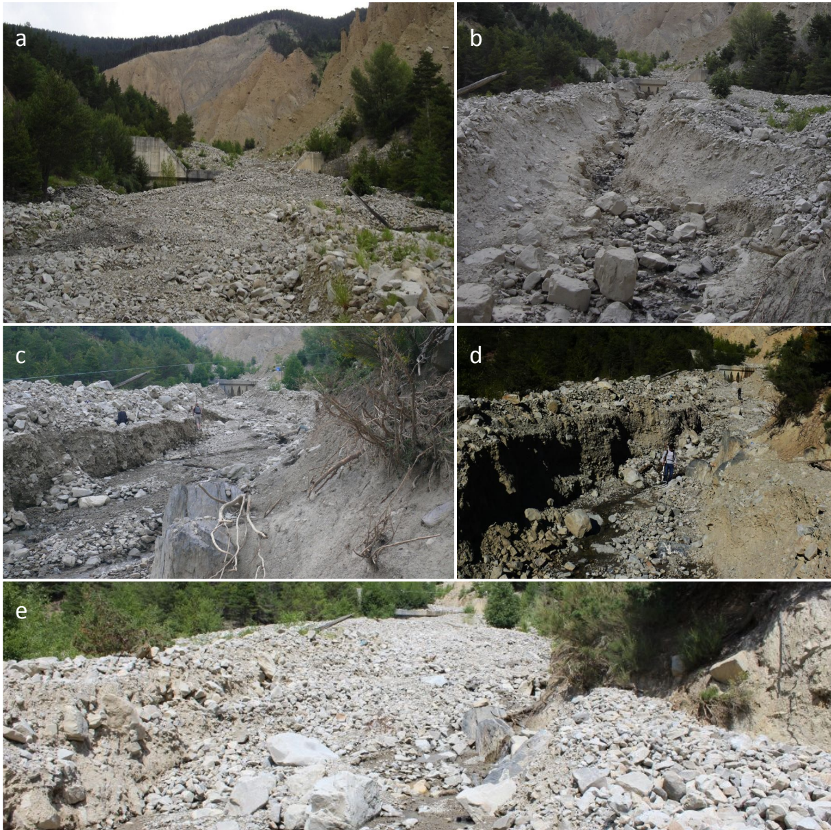
Figure 8. Pictures (from G. Piton) taken on the S_1 stations over 6 years a) channel filled in June 2009, b) channel deeply incised in July 2011, c) channel widened and partially refilled in June 2014 (person for scale), d) channel further incised October 2014 (person for scale), e) channel refilled in July 2014 (pictures from the authors)
