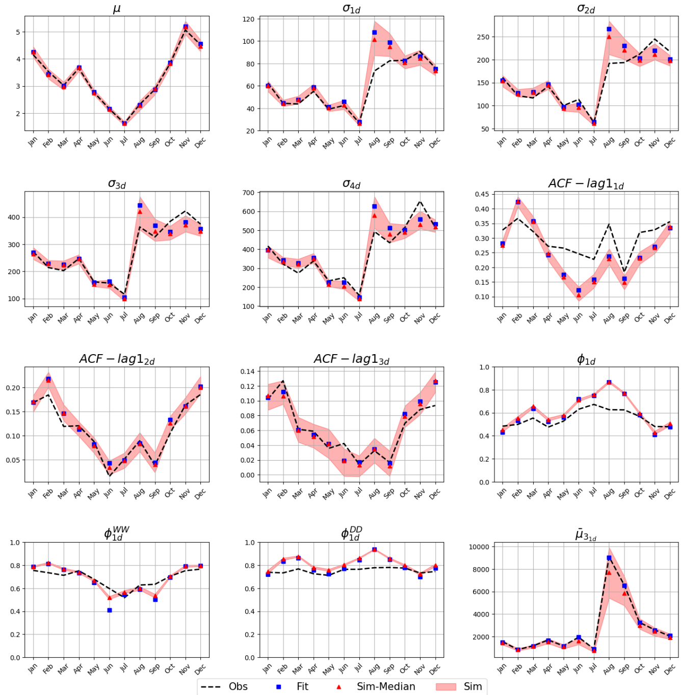
Figure 3. Validation plot comparing the observations (dashed line), the fitted (blue squares) and the simulated (red triangles and red shading) statistics, where \mu refers to rainfall average, \sigma to the variance, ACF-lag1 to the autocorrelation of lag one, \Phi to the probability of dry period, \Phi^{WW} to the probability of having two consecutive wet periods, \Phi^{DD} to the probability of having to consecutive dry periods and (\bar{\mu}_3) to the skewness. The subscripts (1d, 2d, etc.) represent the level of aggregation (in days) at which the statistic was computed. The shading shows the range between the 5% and the 95% percentiles. This figure is generated with the Analysis python class.
