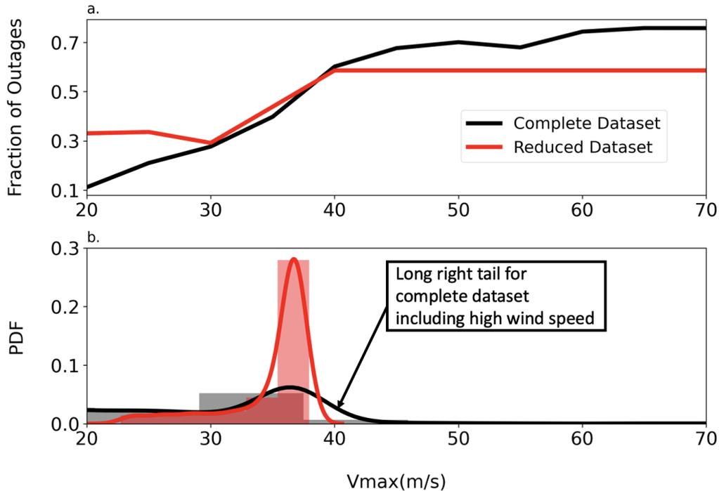
**Figure 10.** (a) Partial dependence of wind speed on power outages. (b) Distribution of wind speed in the complete and reduced dataset. Random Forest model does not extrapolate for the wind speeds and outages not in the range of training data.
