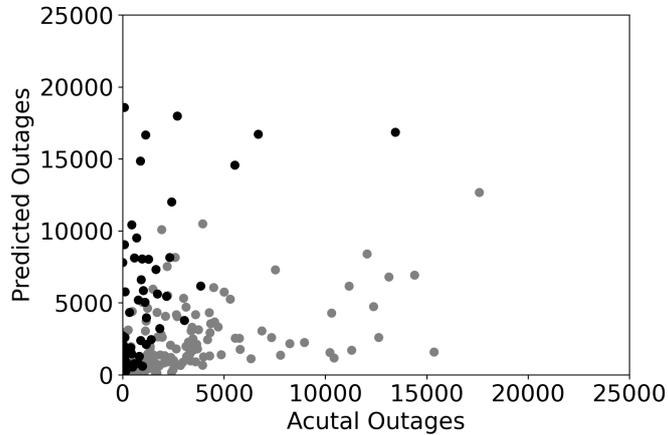
**Figure 9.** Outage predictions on 20% holdout test data using Negative Binomial GAM outage model. Black dots represent the cities with predicted outages larger than the number of customers. Grey dots represent the cities with predicted outages less than or equal to number of customers.
