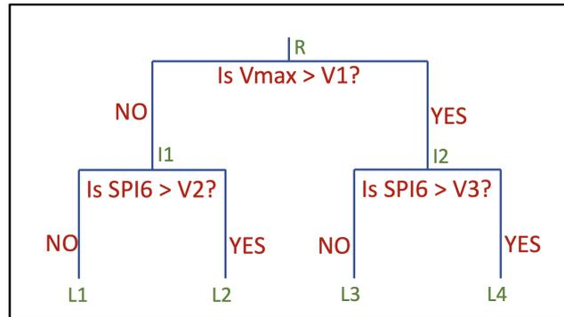
**Figure 6.** Example of a simple decision tree with two input features: maximum wind speed ( $V_{max}$ ) and precipitation ( $SPI6$ ) to predict outages. Split at the root node ( $R$ ) is done with  $V_{max}$ . Thus, if the wind speed value is greater than the value  $V1$ , the points will belong to the right interior node ( $I2$ ) otherwise they belong to the left node. Similarly, interior nodes are further divided into leaf nodes  $L1$ ,  $L2$ ,  $L3$ , and  $L4$  using values of  $SPI6$ .
