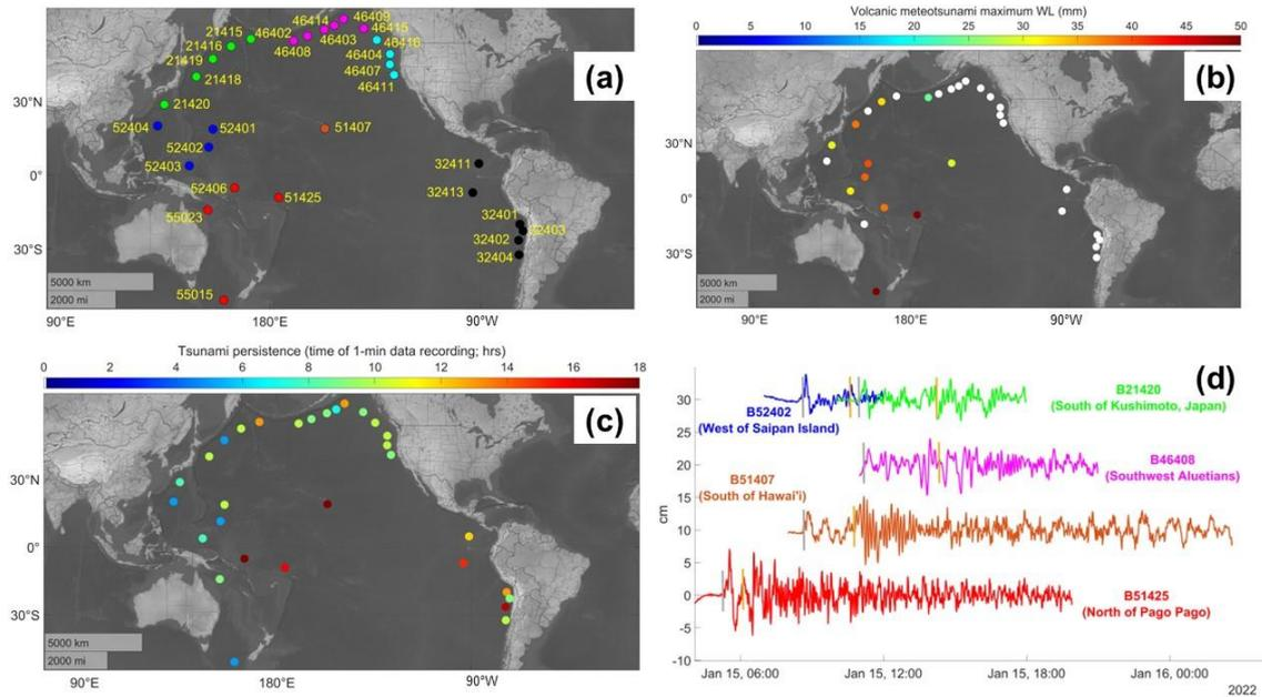
321 **Figure 2** Pacific deep-water NDBC buoys used to detect the VMT and marine tsunami of the Tonga event. (a)
