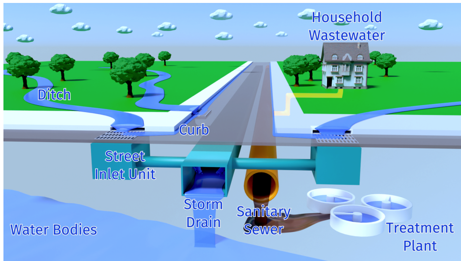
Figure 1. A schematic of an urban drainage system adapted from Town of Gilbert, AZ (2022).
