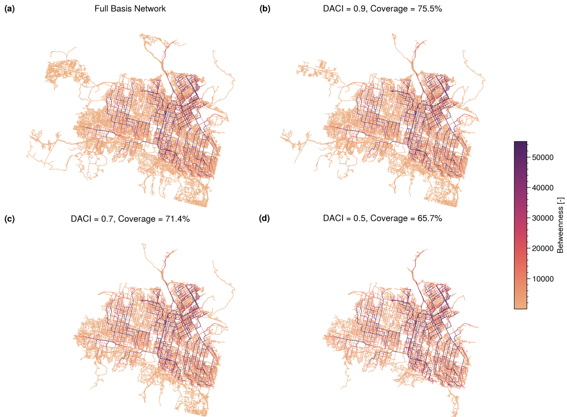
Figure 11. Three different BUSNs estimated for San Fernando Valley with different three different drainage discharge capacities; (a) Full street network, (b) 0.9, (c) 0.7, and (c) 0.5.
