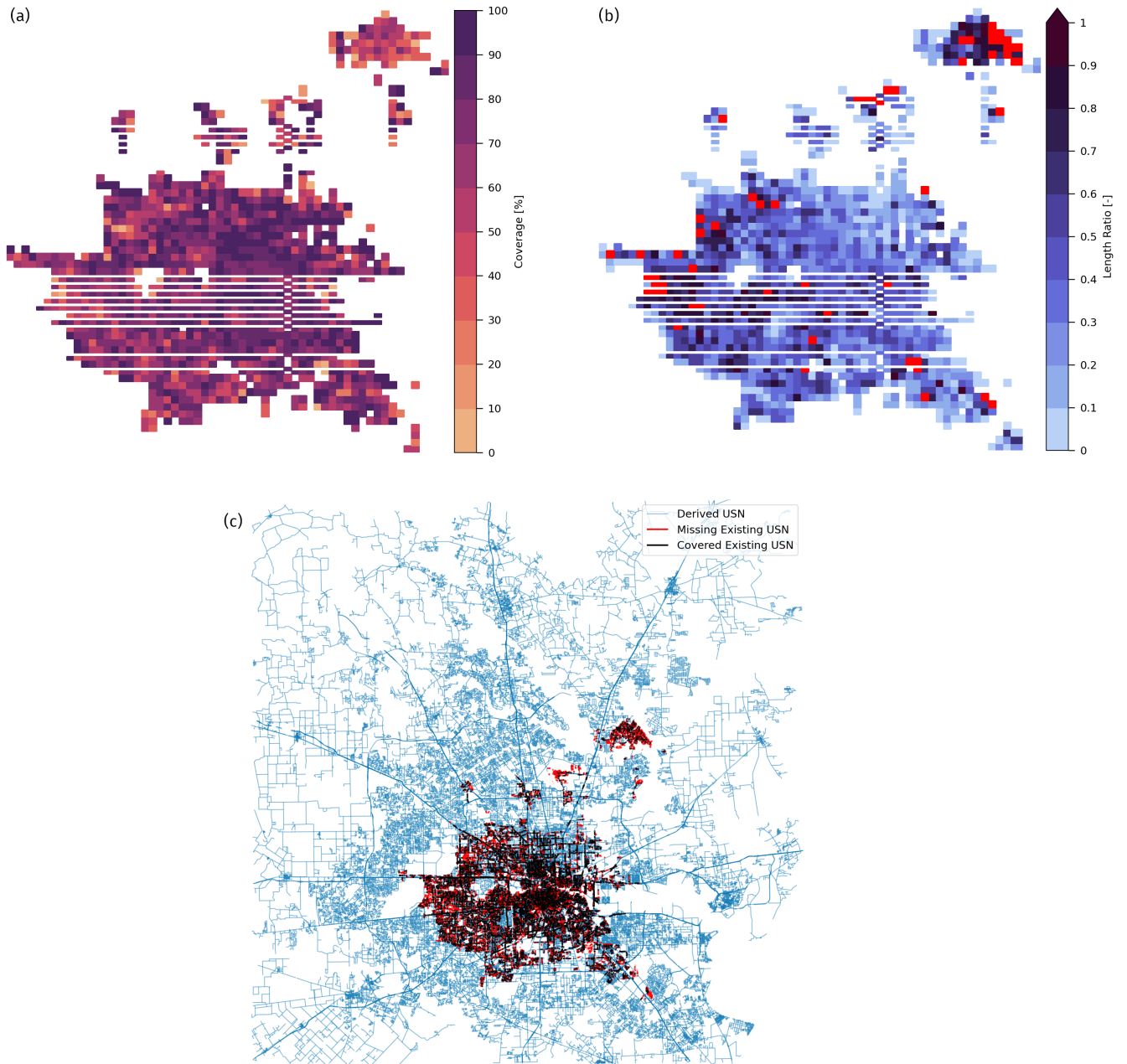
Figure 13. Results for the Houston case. (a) The coverage percentage and (b) length ratio maps at 1 km resolution where the red pixels indicate the areas with poor street data quality. The white background pixels are grid cells that do not contain street and/or existing BUSN elements. (c) compares the estimated BUSN with the existing BUSN using 0.8 DACI.
