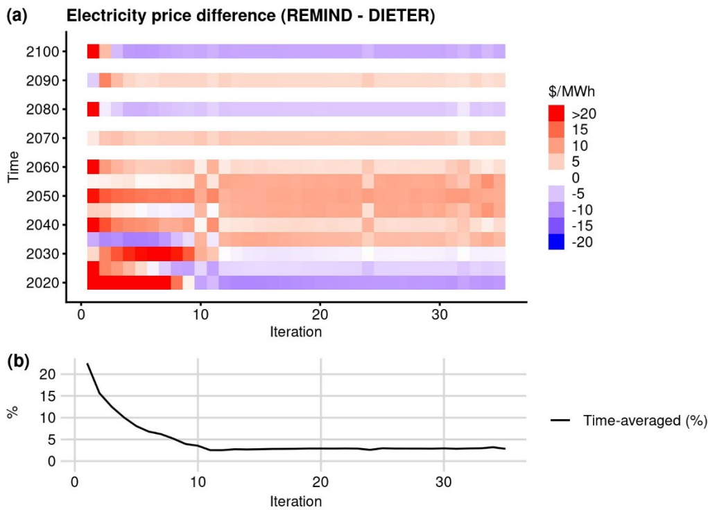
Figure 4: Annual average electricity price convergence behavior of a coupled run for Germany under a “proof-of-concept” baseline scenario. (a): the difference between the annual electricity price time series of REMIND and the annual average electricity price time series in DIETER as a function of coupled iteration. (b): the interannual average of the differences in (a) as a share of REMIND price. Due to the interannual intertemporal nature of REMIND, in (a) the price difference can appear to have oscillatory components, obscuring the visual assessment of convergence. As a result, we show the trend of price convergence over iterations more clearly in panel (b) by taking the temporal average of the price differences. The REMIND price in both plots is a running average of three neighboring time periods to visually smooth out oscillations.
