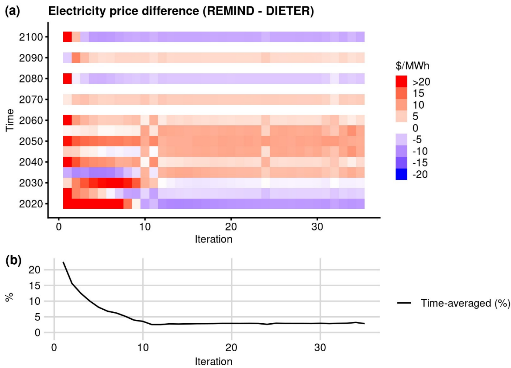
Figure 4: Annual average electricity price convergence behavior of a coupled run for Germany under a “proof-of-concept” baseline scenario. (a): the difference between the annual electricity price time series of REMIND and the annual average electricity price time series in DIETER as a function of coupled iteration. (b): the interannual average of the differences in (a) as a share of REMIND price. Due to the interannual intertemporal nature of REMIND, in (a) the price difference can appear to have oscillatory components, obscuring the visual assessment of convergence. As a result, we show the trend of price convergence over iterations more clearly in panel (b) by taking the temporal average of the price differences. The REMIND price in both plots is a running average of three neighboring time periods to visually smooth out oscillations.
