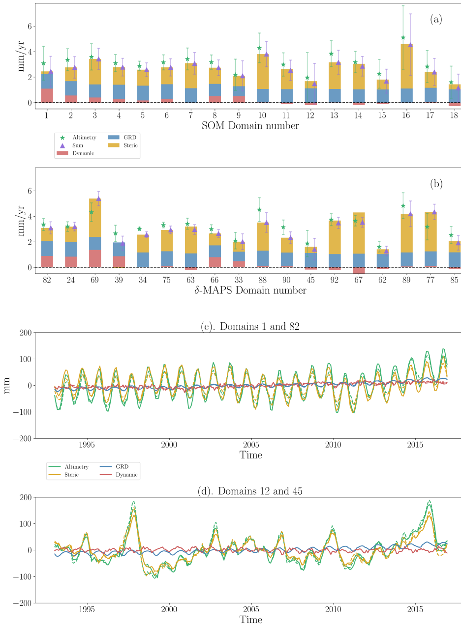
Figure 4. Sea-level budget trends (mm/yr) for (a) SOM and (b) \delta -MAPS domains, and (c,d) time series for two example domains, where solid and dashed lines indicate SOM and \delta -MAPS time series, respectively . Location of each domain is shown in Figure 2 (domain numbers in magenta for \delta -MAPS). For comparison \delta -MAPS domains are matched to the SOM domains, for example SOM domain 12 to \delta -MAPS domain 45. For time series, solid and dashed lines Error bars indicate SOM and \delta -MAPS time series, respectively the 1-sigma uncertainty of the trend . Time series for all SOM domains and for the 18 \delta -MAPS domains in (b) are shown in Supplementary Figure B4. An interactive budget map is available at https://carocamargo.github.io/portfolioresources/portfolio-1-regional-SLB-domains/ for both SOM and \delta -MAPS.
