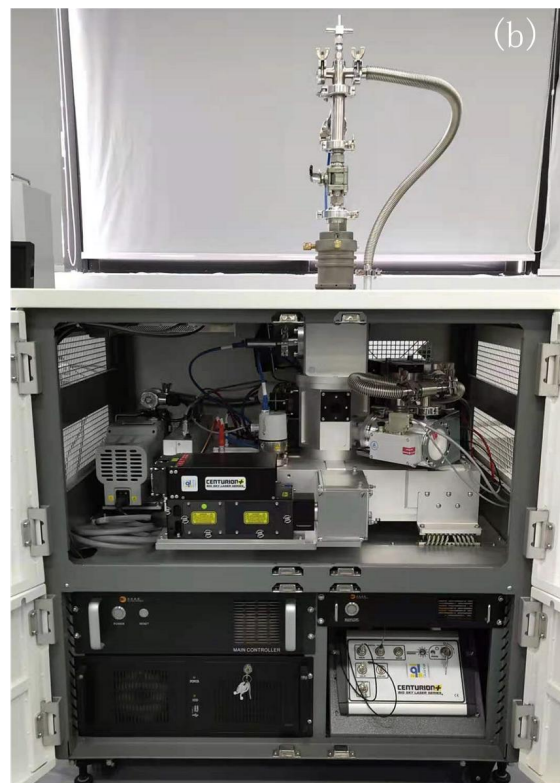
Figure 1: Schematic diagram and photograph of the HP-SPAMS instrument. (a) The aerosol particles were introduced through an APC into an improved aerodynamic lens (ADLs) to focus into a particle beam. A scattering system measured the particle size with two higher power continuous lasers (532nm). Particle chemical components were obtained by bipolar time-of-flight mass spectrometry analysis of ions derived from a pulsed laser (266nm) ablation/ionization of particles. (b) The instrument's main body was placed in the upper part of the frame, and the lower part was composed of the power supply, control unit, and pump.
