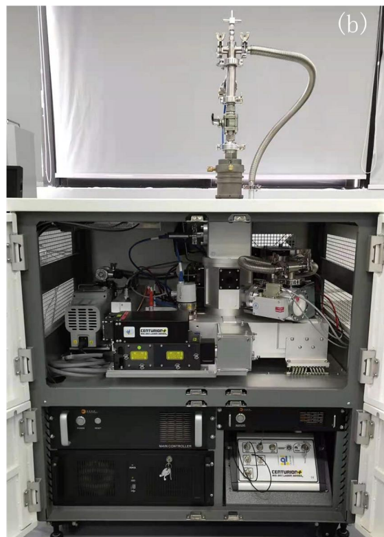
500 Figure 1: Schematic diagram and photograph of the HP-SPAMS instrument. (a) The aerosol particles were introduced through an APC into an improved aerodynamic lens (ADLs) to focus into a particle beam. A scattering system measured the particle size with two higher power continuous lasers (532nm). Particle chemical components were obtained by bipolar time-of-flight mass spectrometry analysis of ions derived from a pulsed laser (266nm) ablation/ionization of particles. (b) The instrument's main body was placed in the upper part of the frame, and the lower part was composed of the power supply, control unit, and pump.
