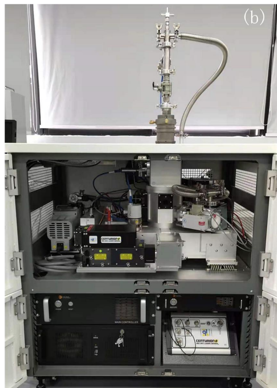
445 Figure 1: Schematic diagram and photograph of the HP-SPAMS instrument. (a) The aerosol particles were introduced through an APC into an improved aerodynamic lens (ADLs) to focus into a particle beam. A scattering system measured the particle size with two higher power continuous lasers (532nm). Particle chemical components were obtained by bipolar time-of-flight mass spectrometry analysis of ions derived from a pulsed laser (266nm) ablation/ionization of particles. (b) The instrument's main body was placed in the upper part of the frame, and the lower part was composed of the power supply, control unit, and pump.
