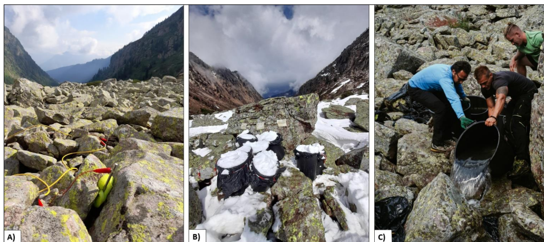
191 192 Figure 2: A) Electrodes inserted between the boulders using sponges soaked with saltwater to improve the contact resistances of the 193 ERT surveys; B) 10 bins placed at the selected injection point in early spring 2022, filled with snow and covered with nylon sheets 194 pierced at their center to collect rainwater; C) Injection of 800 liters of salt water into the subsoil system.
