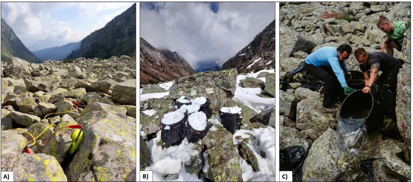
171 172 Figure 2: A) Electrodes inserted between the boulders using sponges soaked with saltwater to improve the contact resistances of the 173 ERT surveys; B) 10 bins placed at the selected injection point in early spring 2022, filled with snow and covered with nylon sheets 174 pierced at their center to collect rainwater; C) injection of 800 liters of salt water into the subsoil system.
