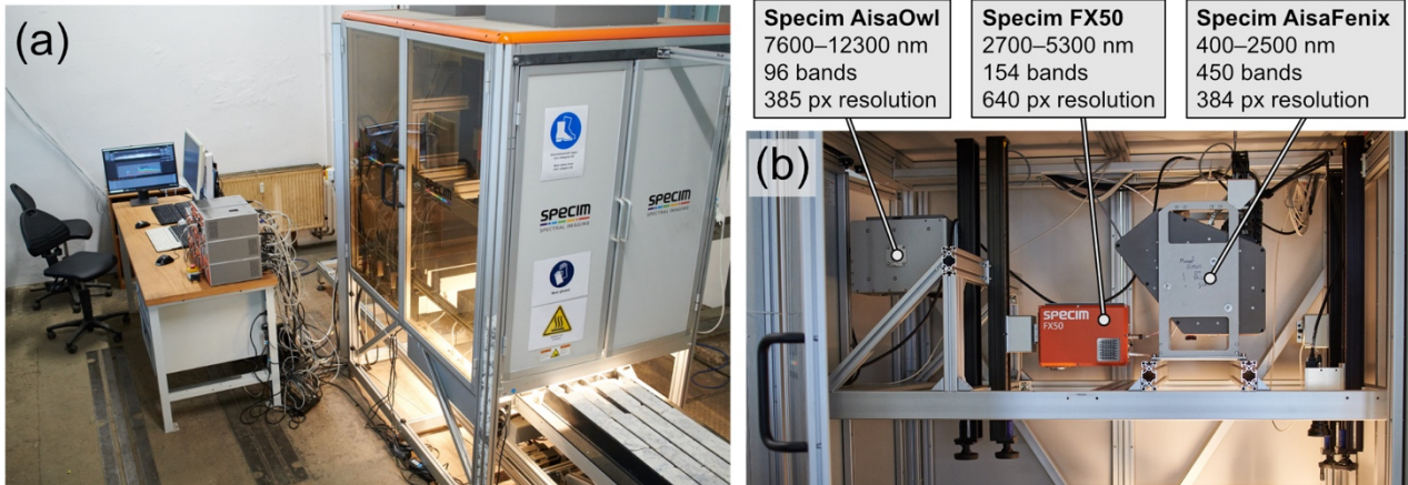
Figure 4. (A) Specim Sisurock hyperspectral drill core scanner with (B) mounted sensors in the visible to near-infrared and short-wave infrared (VNIR-SWIR), mid-wave infrared (MWIR), and long-wave infrared (LWIR) range.
