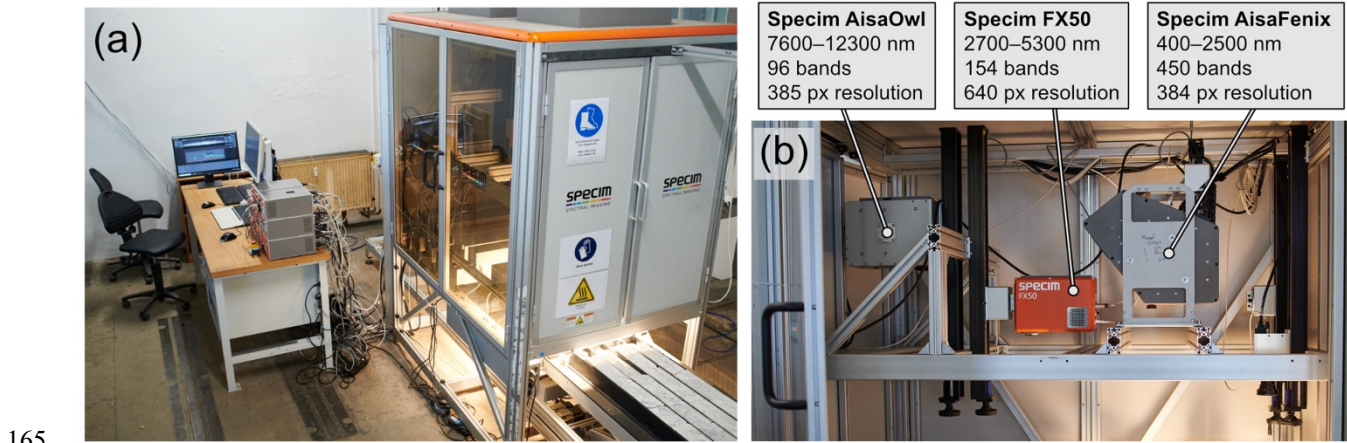
Figure 4. (A) Specim Sisurock hyperspectral drill core scanner with (B) mounted sensors in the visible to near-infrared and short-wave infrared (VNIR-SWIR), mid-wave infrared (MWIR), and long-wave infrared (LWIR) range.
