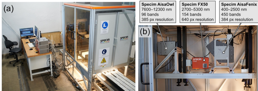
240 Figure 4. (A) Specim Sisurock hyperspectral drill core scanner with (B) mounted sensors in the visible to near-infrared and short-wave infrared (VNIR-SWIR), mid-wave infrared (MWIR), and long-wave infrared (LWIR) range.
