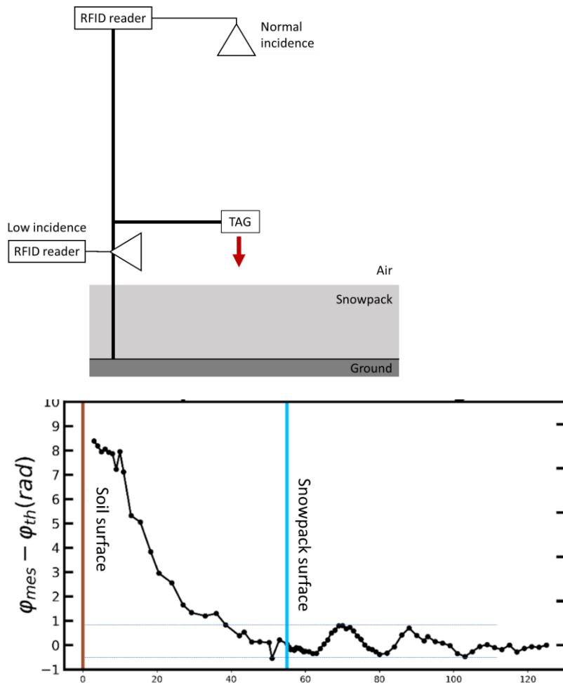
In another experiment, we have removed a thin layer of snow from the ground, with tags placed at different locations. As a consequence, the phase varied between +1 to -2 rad (3 rad of amplitude). It is coherent with the changes expected from a simple 3-ray model.
