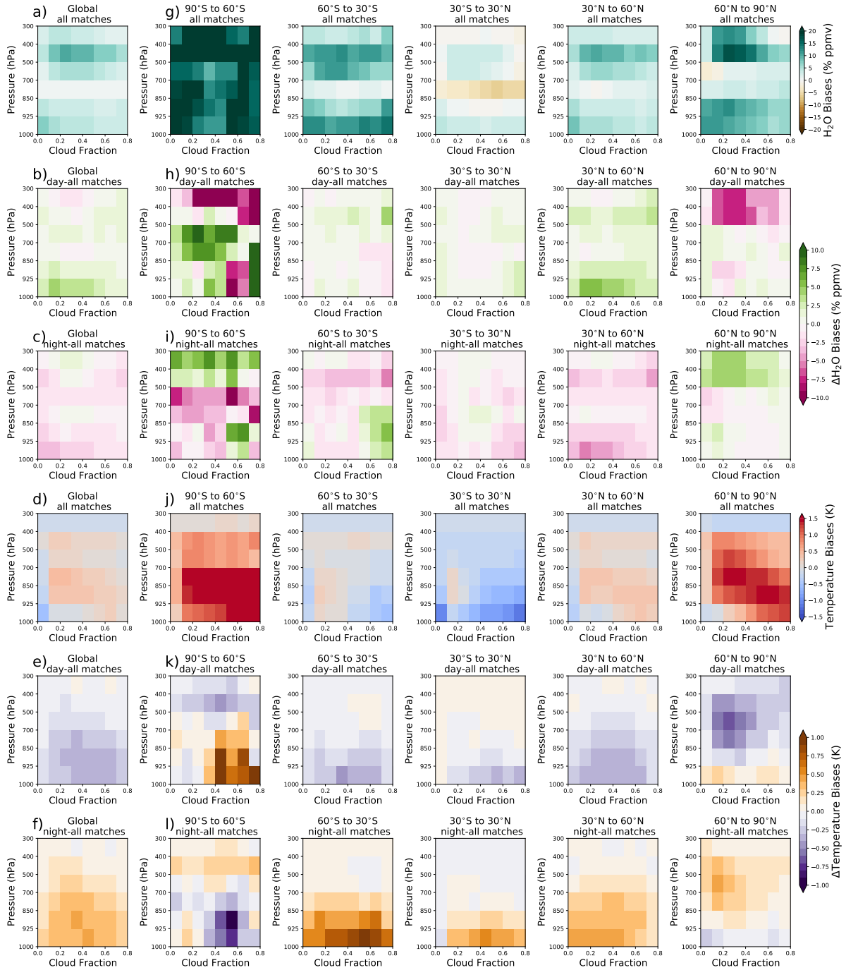
Figure 11. Cloud fraction effects on IMS biases relative to ARSA radiosonde water vapour and temperature profiles. Results here are broken down into; global water vapour and temperature biases (a, d), daytime differences to global biases (b, e), night-time water vapour and temperature bias differences (c, f), and biases calculated for five broad latitudinal bands (g, j) and the day and night-time differences (h, i & k, l respectively).
