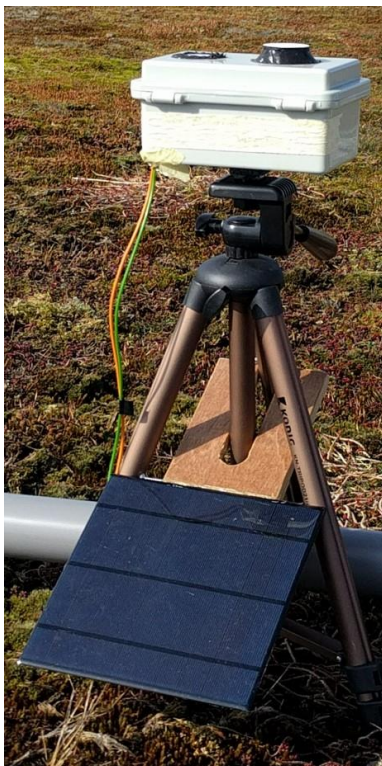
124 Figure 2: FROST with solar panel mounted on a camera tripod.
