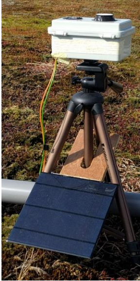
134 Figure 2: FROST with solar panel mounted on a camera tripod.
