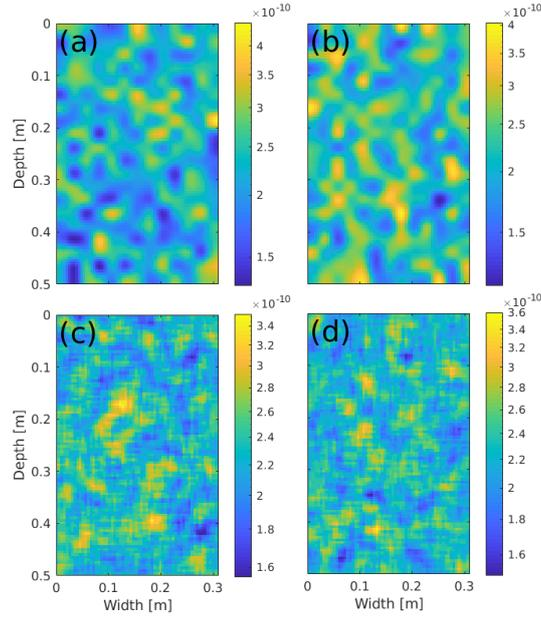
**Figure B1.** The distribution of the intrinsic permeability  $\kappa$  [ $\text{m}^2$ ] used for the sensitivity analysis of the Bauters' paradox. The distributions satisfy: (a)  $\kappa_{max}/\kappa_{min} \approx 3.40$ , (b)  $\kappa_{max}/\kappa_{min} \approx 3.48$ , (c)  $\kappa_{max}/\kappa_{min} \approx 2.28$ , (d)  $\kappa_{max}/\kappa_{min} \approx 2.42$ . Intrinsic permeability values are colour-coded according to the colour bar on the right.
