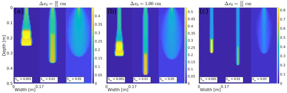
**Figure 2.** Snapshots of the saturation field for various  $\Delta x_0$  for initially dry ( $S_{in} = 0.001$ ), a medium dry ( $S_{in} = 0.01$ ) and a wet ( $S_{in} = 0.05$ ) porous material. The moisture profiles for (a)  $\Delta x_0 = \frac{10}{12}$  cm, (b)  $\Delta x_0 = 1.00$  cm and (c)  $\Delta x_0 = \frac{12}{10}$  cm are shown at 30, 30 and 20 minutes, respectively. Saturation values are colour-coded according to the colour bar on the right.
