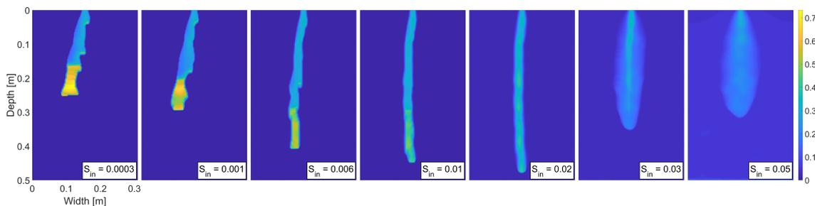
**Figure 4.** Snapshot of the saturation field at 25 minutes for seven different values of the initial saturation. Saturation values are colour-coded according to the colour bar on the right. Initial saturation of the medium increases from left to right.
