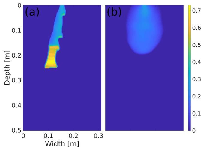
**Figure 9.** The role of the geometric mean of the hydraulic conductivity and the scaling of the retention curve. Snapshot of the saturation field for (a) the semi-continuum model and (b) without utilizing the geometric mean of the hydraulic conductivity and the scaling of the retention curve at  $t = 25$  minutes for  $S_{in} = 0.0003$ . Saturation values are colour-coded according to the colour bar on the right.
