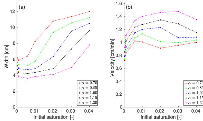
**Figure B4.** The effect of the retention curve on the flow regime. The width (a) and the velocity (b) of the finger (or wetting front) at  $t = 25$  minutes is plotted against the initial saturation for five different values of parameter  $\alpha$ . The averages of four different distributions of the intrinsic permeability are plotted.
