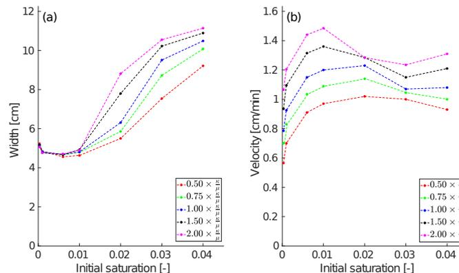
**Figure B2.** The effect of the intrinsic permeability and dynamic viscosity on the flow regime. The width (a) and the velocity (b) of the finger (or wetting front) at  $t = 25$  minutes is plotted against the initial saturation for five different values of  $b \cdot \frac{\kappa}{\mu}$ . The average of four different distributions of the intrinsic permeability is plotted.
