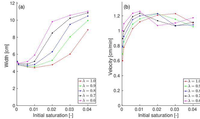
**Figure B3.** The effect of the relative permeability on the flow regime. The width (a) and the velocity (b) of the finger (or wetting front) at  $t = 25$  minutes is plotted against the initial saturation for five different values of parameter  $\lambda$ . The average of four different distributions of the intrinsic permeability is plotted.
