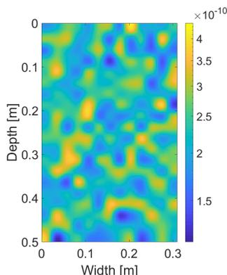
**Figure 3.** The distribution of the intrinsic permeability  $\kappa$  [ $\text{m}^2$ ], which satisfies  $\kappa_{max}/\kappa_{min} \approx 4$ . Intrinsic permeability values are colour-coded according to the colour bar on the right.
