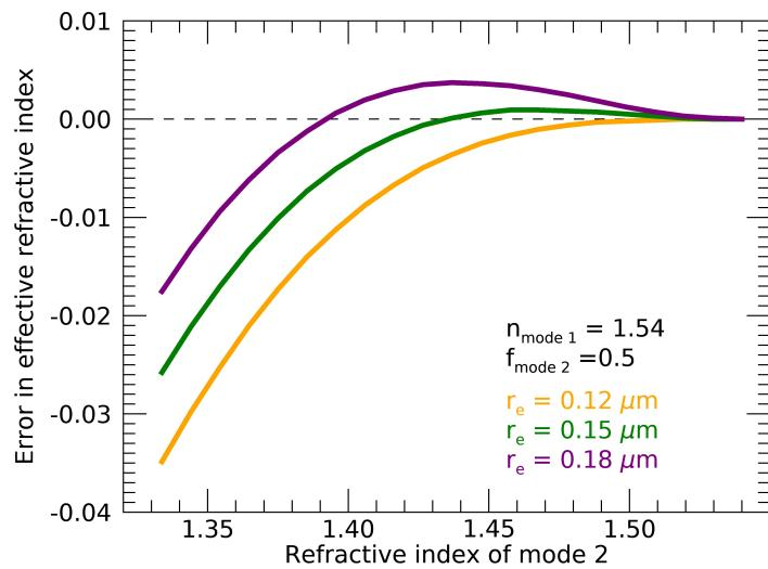
**Figure S2.** Error in effective refractive index of a two-mode aerosol mixture from applying the volume fraction mixing rule as a function of the refractive index of one of the modes. The other mode is assumed to have a refractive index of 1.54. An equal fraction of the two modes is assumed. Results are shown for aerosols with size distributions with a effective radius of 0.12 (orange), 0.15 (green) and 0.18 (*purple*)  $\mu\text{m}$ .
