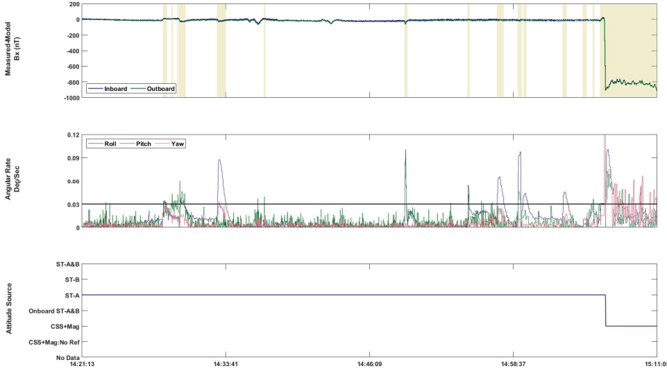
Figure 3: (Top) Residuals for the B_x component for inboard (blue) and outboard (green). Areas marked in yellow represent any point where the rotation rate exceeded 0.03 deg/sec or the attitude solution was not generated by at least one star-tracker camera. The various flags applied to the sensor data. Gray represents points where the angular rotation rate of the spacecraft exceeds 0.03 degrees/sec. Pink represents places where the attitude solution was not generated by at least one star-tracker camera or where it has been longer than ten seconds since the last attitude signal has been received or it will be longer than ten seconds until the next attitude signal will be generated. (Middle) The angular rotation rate corresponding to the data in the top plot. (Bottom) The seven potential attitude sources for the data which have significantly different accuracies of solution. The potential errors in the attitude solution derived from CSS versus one of the star-tracker cameras is clearly shown by the transition from ST-A (star tracker A only) to CSS (coarse sun sensor).
