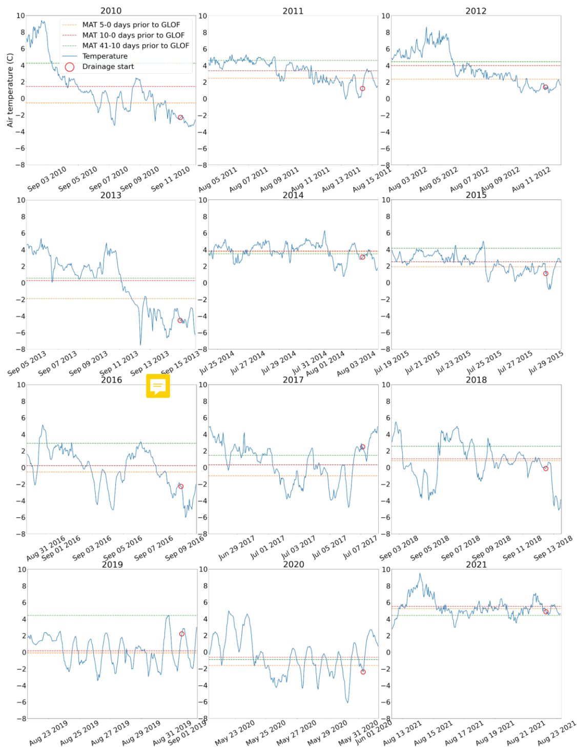
Figure 5. Plot of hourly temperature measurements from 10 days prior to the drainage event from KAN L. Green line shows the mean air temperature (MAT) 41-10 days prior to the drainage, red line shows MAT 10-0 days prior, and orange line MAT 5-0 days prior to drainage. Red circle denotes the start of the GLOF and for the 2018 event the circle is larger due to uncertainty about the timing.
