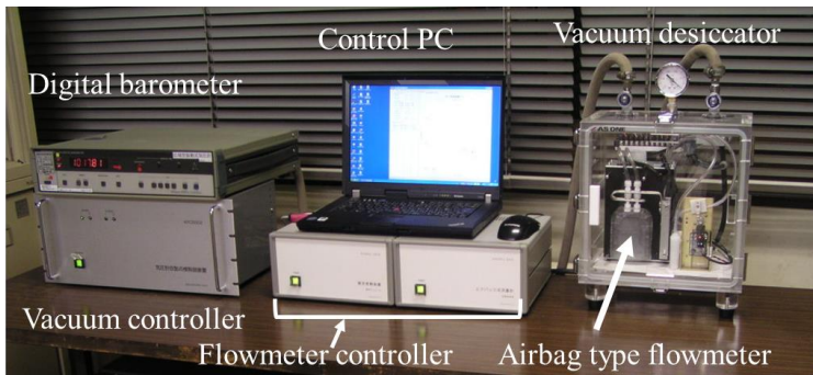
Figure 4: Actual appearance of automated measurement system of the pump efficiency for the ECC ozonesonde.
