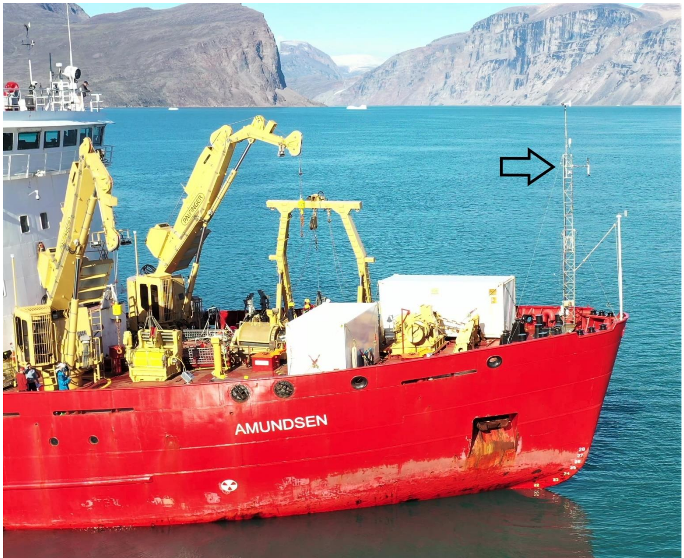
Fig. A1: The measurement tower at the bow of the ship with anemometer, temperature sensor, and air inlet mounted on the truss approximately where the arrow is pointing. The GPS was fixed at the lower end of the truss. Photo credit to David Cote (DFO, Canada).
