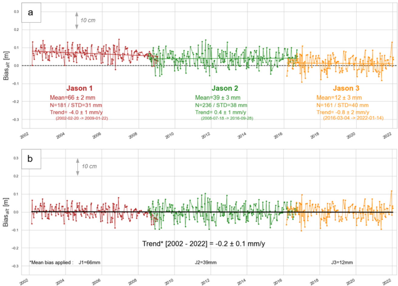
Figure 9. (a) Altimeter bias time series at the comparison point for Jason 1 (red), Jason 2 (green) and Jason 3 (orange) track #162. / (b) Altimeter bias time series after applying mean biases found in this study (i.e. -66mm for J1, -39mm for J2 and -12mm for J3). The black line represents the resulting trend compute over the whole Jason period [2002-2022].
