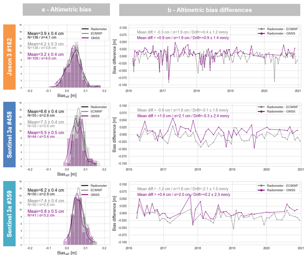
Figure 6. Altimetric bias at the comparison point according to different wet tropospheric models and for 3 altimetric tracks: the Jason 3 (orange) track #162, the Sentinel-3a tracks #458 (dark blue) and #359 (light blue) / (a) Altimetric biases distribution as a function of the wet tropospheric delay from the radiometer (black), the ECMWF model (grey) and the GNSS stations (purple). / (b) Bias time differences from the radiometer solution with respect to the ECMWF model (grey) and GNSS stations (purple).
